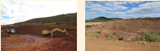
Fig. 1: Laterites in the mine Barro Alto (Anglo American), federal state Goiás, Brazil. Left: Fresh limonite. Right: Stockpile. Source: BGR.
