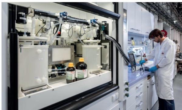
Preliminary investigations into the concentration of geothermal brines with a membrane distillation test cell.
