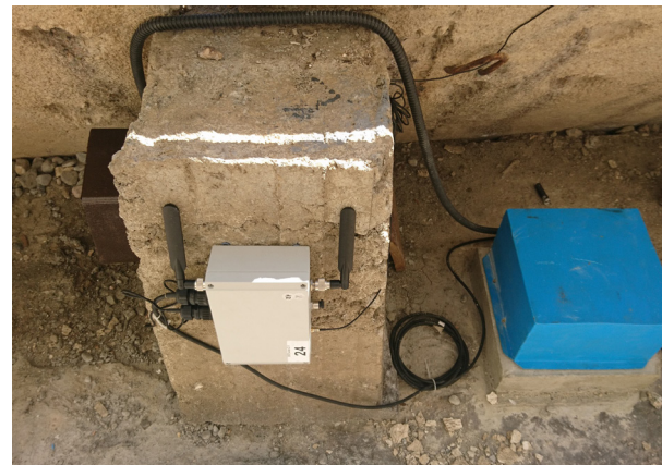
Installation of seismic sensors and the real-time data transmission system using WLAN technology.
